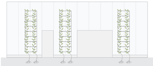
Ground based and trellis-supported green facade
